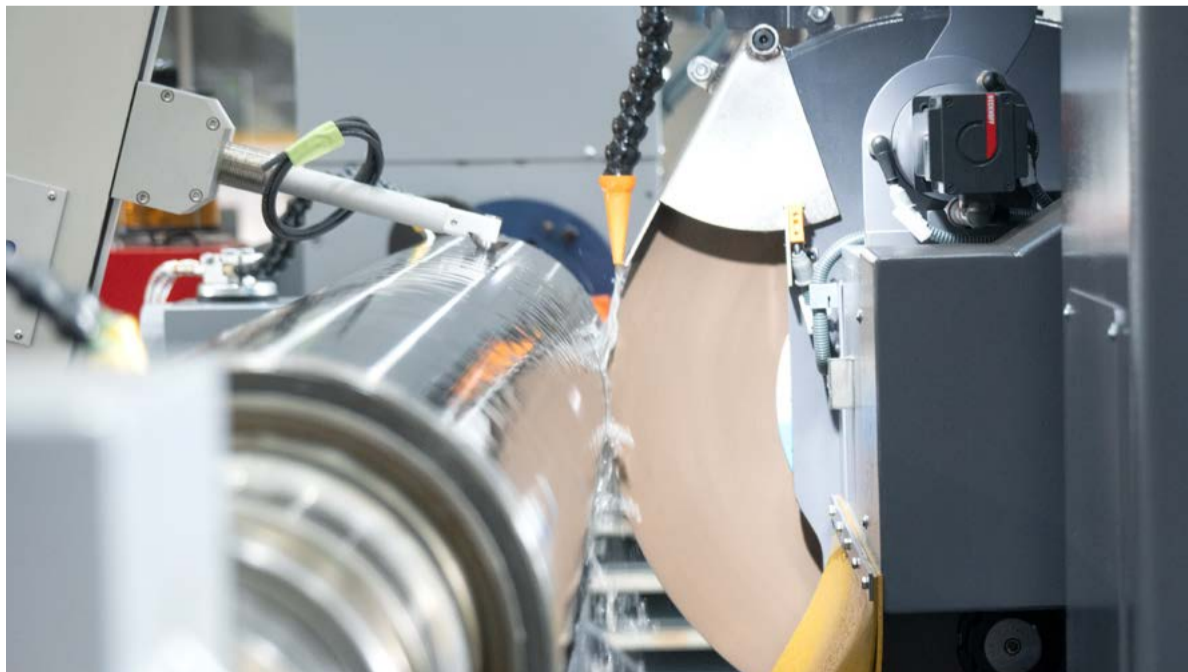
Modern coating processes require extremely smooth film surfaces for optimum coating results. Herkules measuring and testing technology ensures smooth, homogeneous roughness across the entire roll
