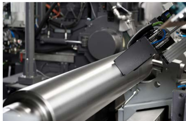
The Roll Surface Inspection System (RSIS) for the automatic detection of surface defects on the roll
